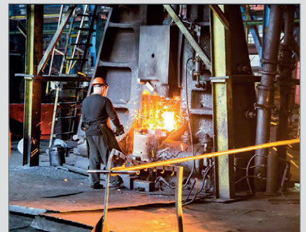
Metal Forming: Fabreeka pads used to greatly diminish impact shock from forging hammers and presses
