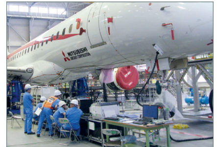
Aircraft Testing: Fabreeka Soft Support System used to float aircraft for ground vibration testing
